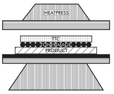
Note: Let product rest for 5-10 seconds on the HeatPress before stripping the backing paper! If you take it off the HeatPress strip immediately. Tip: To flatten down fabric nap in light image areas re-press with Release Paper or slap the areas while still hot/warm.
